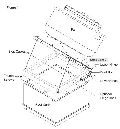
6. Rotate the lower hinge until parallel with the upper hinge. If cap has factory holes that line up with hinge holes, go to Step 7. If cap does not have matching holes from the factory, mark the hole locations in the curb and drill a 5/16 inch hole at each location. Reference Figure 4.
