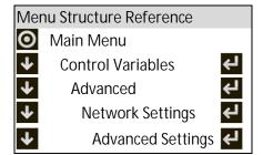
Additional settings can be accessed in the BACnet Advanced Settings menu including BACnet Broadcast Management Device (BBMD) configuration, relinquish default settings, Change of Value (COV) increments and restoring binary text values.
