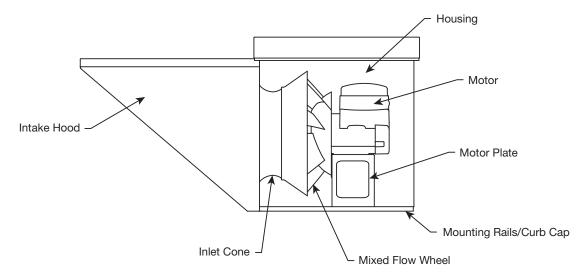
**NOTE:** Fan size 18 and larger have additional internal structural supports.
