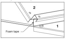
3. Use the self-tapping sheet metal screws to mount second panel
