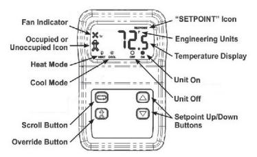
**Override Button Function** - The display shows a person in the lower left corner of the display at all times. If the person is solid, the unit is operating in occupied mode. If it is an outline of the person, the unit is in unoccupied mode. Pushing the Override button when the unit is in unoccupied mode temporarily overrides the sequence to Occupied mode for a period of 1 to 4 hours (adjustable at the unit microprocessor).
