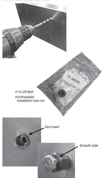
Turn bolt to collapse the nut insert
