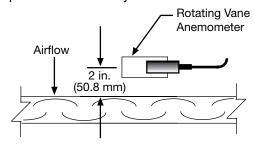
Calculate the average velocity for the filter.
