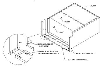
To allow for ease of cleaning, caulk the external seams with NSF Approved silicone caulk (GE SCS1009, or its equivalent). The caulk is not provided.
