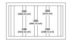
For a nominal filter size of 20 x 16, the conversion factor is 1.90 Imperial (.177 Metric)
