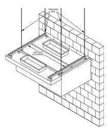
Uni-strut (supplied by others) supporting the hood may be cantilevered over the end of the hood where applicable. Utilizing the external supply plenum's hanger brackets, securely fasten to the uni-strut.
