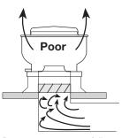
Dampers must open fully. Use motorized dampers in low airflow applications to reduce losses.
