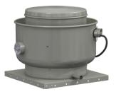
Wheel - Backward-inclined, non-overloading centrifugal wheel is utilized to generate high-efficiency and minimal sound. Wheel cones are carefully matched to the venturi for maximum efficiency. Each wheel is statically and dynamically balanced, for long life and quiet operation.
