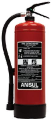
The F-CLASS Liquid Agent Fire Extinguisher (European) provides dependable and superior backup to an automatic fire suppression system. This extinguisher is designed to protect commercial cooking equipment with a low pH fire extinguishing agent that provides rapid fire suppression and securement of hot fuels such as combustible vegetable oils or animal fats.
